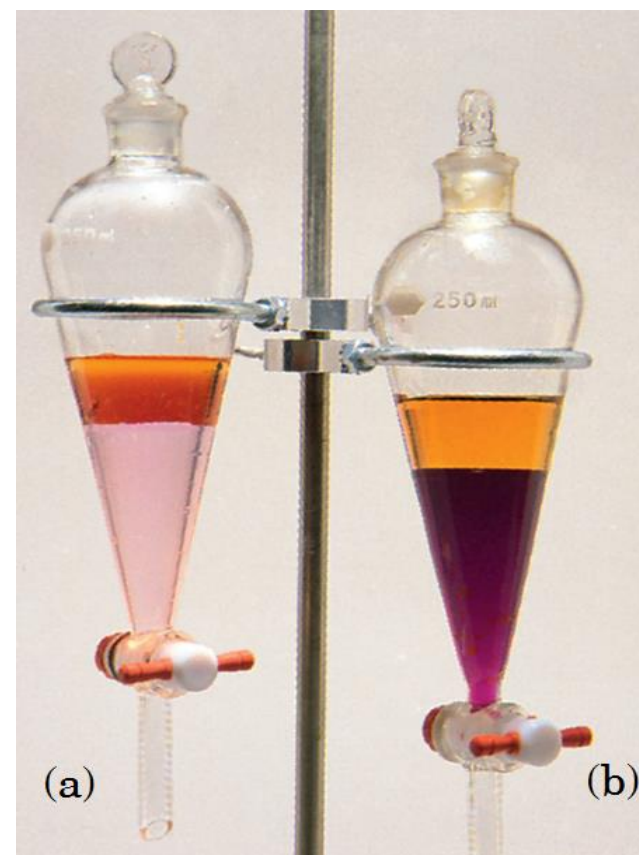
Fig. 14.13. (a) I_2(aq) on CCl_4 in a separatory funnel. (b) After shaking.
